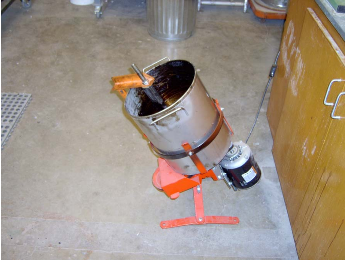
FIGURE 21 Bucket mixer used for mixing CIR samples.
