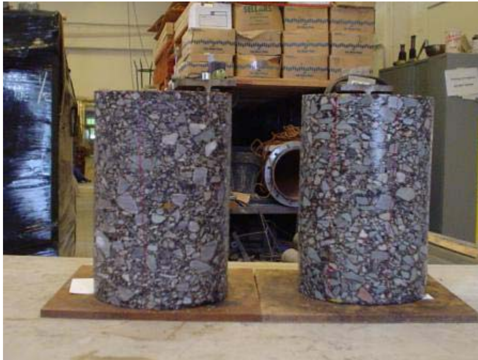
FIGURE 24 Test specimens for dynamic modulus testing.
