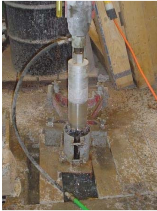
FIGURE 22 Sample being cored to required test diameter.
